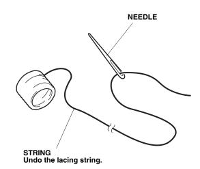
5. Starting at the back of the left spoke, lace the string through the holes of the steering wheel cover from the inside. Leave approx. 100 mm (3.93 in.) of string at the end. This will be used to tie the string when finished.
