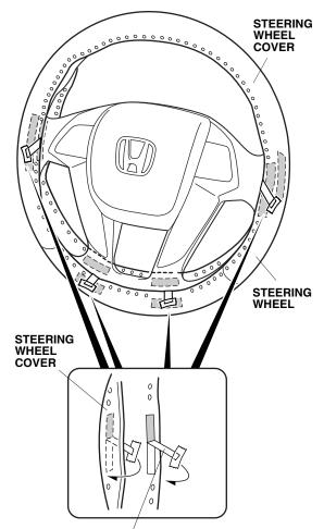
8 ADHESIVE BACKINGS Peel back the adhesive backings and temporarily attach them to the front of the steering wheel cover with masking tape. 4. Thread the string through the needle as shown.
