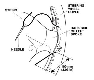
6. Tightly lace the string twice through the holes directly above the left spoke as shown.
