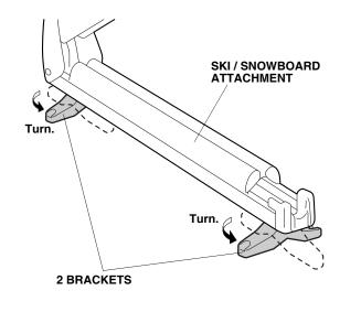
4. Using a wrench, install the ski / snowboard attachment to the front crossbar with four bolts, four collars, and two brackets.
