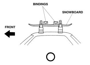
11. If the bindings cannot be positioned between the front and the rear attachments, install the the rear binding behind the rear attachment as shown.
