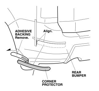
18. Align the corner protector with the masking tape and attach the corner protector to the rear bumper.
