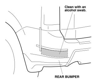
17. Remove the adhesive backing from the corner protector. Check the back of the corner protector for the correct orientation.
