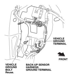
38. Route the back-up sensor harness toward the rear of the vehicle, and secure it to the vehicle harness with three wire ties.
