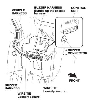
Loosely secure the buzzer harness to the vehicle harness with one wire tie.
