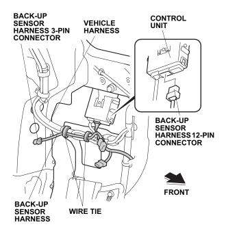
Route the back-up sensor harness 3-pin connector as shown and secure it to the vehicle harness with two wire ties loosely secured in step 29 and 30. 34. Unplug the vehicle 23-pin connector, and plug the back-up sensor harness 23-pin connector to the vehicle 23-pin connector as shown.
