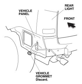
40. Route the back-up sensor harness through the vehicle grommet hole, and install the back-up sensor harness grommet into the vehicle panel.
