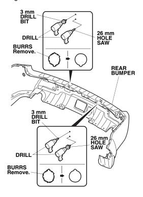
54. Install the two corner sensors in the rear bumper, using one sensor clip for each sensor.
