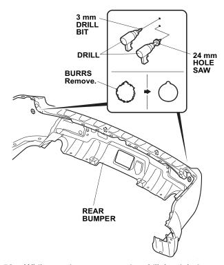
53. While wearing eye protection drill the right inner mark at the upper pierced mark with a 3 mm drill bit. On the left inner mark, drill the lower pierced mark with a 3 mm drill bit. Then drill the two center marks using a 26 mm hole saw. Remove all burrs.
