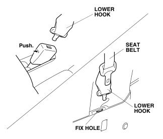
11. Remove the two seat belts from the left third row seat and remove the four bolts fastening the left third row seat to the floor. Remove the left third row seat.
