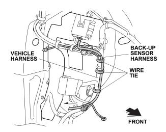
37. Remove the vehicle ground bolt from the vehicle ground terminal. Secure the back-up sensor harness ground terminal to the vehicle ground terminal with the vehicle ground bolt you just removed.
