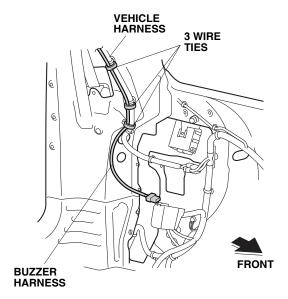
29. Plug the buzzer harness connector to the control unit. Bundle up the excess buzzer harness and loosely secure it to the vehicle harness with one wire tie.
