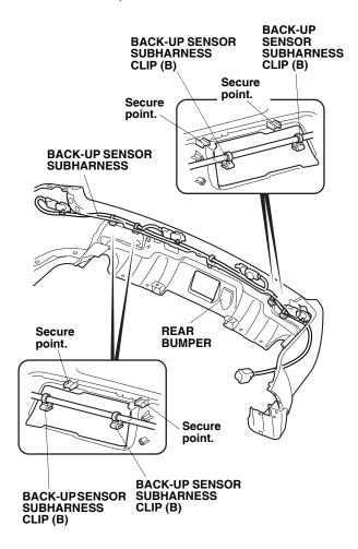
59. Using isopropyl alcohol on a shop towel, clean the area where the harness tape will attach. Secure the back-up sensor subharness to the rear bumper with one harness tape.
