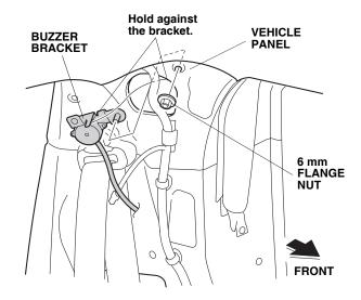
26. Secure the vehicle harness to the buzzer bracket with the offset wire tie as shown.
