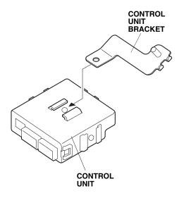
22. Secure the control unit bracket to the vehicle panel with the 6 mm flange nut.
