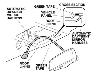
Locate the vehicle 6-pin connector and remove the blue tape. Plug the automatic day/night mirror harness 6-pin connector to the vehicle 6-pin connector.
