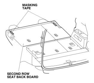
11. Using a felt-tip pen, measure and mark on the masking tape attached in step 10.
