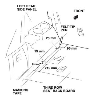
6. While wearing eye protection, drill the two forward marked locations with a 3 mm drill bit and then with a 5 mm drill bit. Drill through the hard board and sheet metal. To prevent damage to the inner vehicle parts, wrap tape around the drill bit 25 mm away from the tip as shown.
