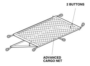
22. Attach five loops on the advanced cargo net to two anchors A (Large), two anchors B (Small) and hook on the third row seat back board.
