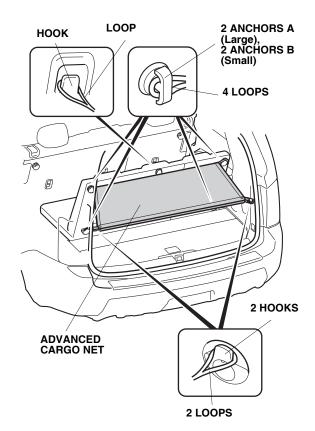
23. Attach two loops on the advanced cargo net to two hooks.
