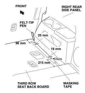
5. Using a felt-tip pen, measure and mark two locations on the masking tape attached in step 3.
