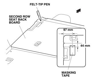
13. While wearing eye protection, drill the marked locations with a 3 mm drill bit and then with a 5 mm drill bit. Drill through the hard board and sheet metal. To prevent damage to the inner vehicle parts, wrap tape around the drill bit 25 mm away from the tip as shown.
