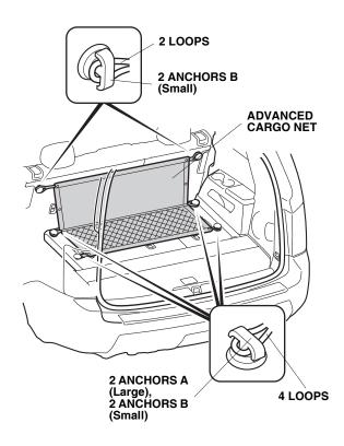
20. Attach six loops on the advanced cargo net to two anchors A (Large) and four anchors B (Small) on the second and third row seat back board.
