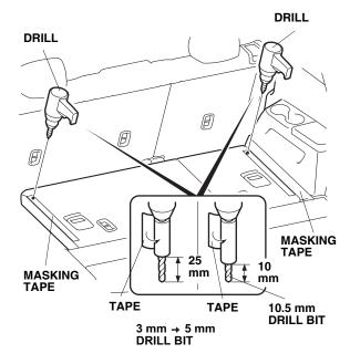
7. Drill at the marked location with a 10.5 mm drill bit. To drill through the hard board only, wrap tape around the drill bit 10 mm away from the tip as shown.
