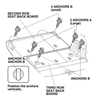
18. Install the four anchors B (Small) on the second and third row seat back board into the holes made in steps 8 and 13.
