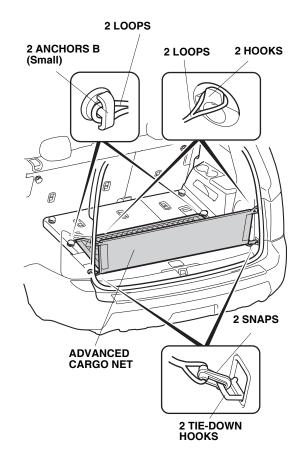
29. Attach two snaps on the advanced cargo net to two tie-down hooks.
