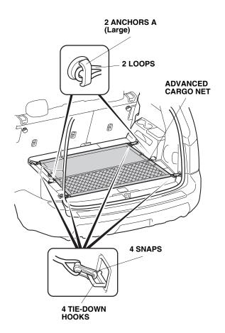
26. Attach four snaps on the advanced cargo net to four tie-down hooks and two loops on the advanced cargo net to two anchors A (Large) on the third row seat back board.
