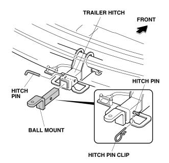
After the first 600 miles (1,000 km) of towing, have your Honda Dealer re-check the tightness of the trailer hitch bolts.
