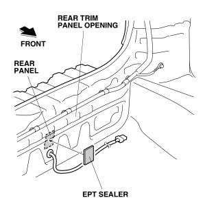
12. Attach the EPT sealer to the rear panel as shown.
