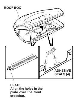
Attach adhesive seals over the unused rear mounting holes along the bottom of the roof box.
