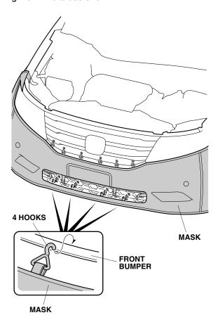
11. Secure the four hooks to the top of the lower grille in the areas shown.
