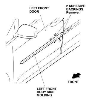
12. Using a rubber roller, apply pressure against the left front body side molding and roll from one end to the other.
