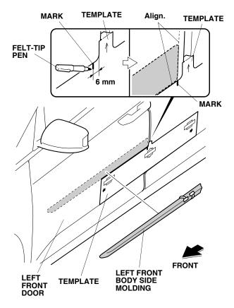
7. Align the left front body side molding with the template and mark on the template, and attach it to the left front door as shown.
