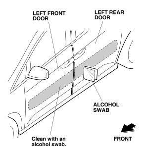
2. Get the template. In the center of the template locate the top and bottom tabs, and fold them back. Insert the folded tabs between the left front door and left rear door.
