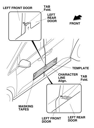
3. Align the template with the character line, and attach the template to the left doors with strips of masking tape as shown.
