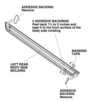
9. Align the left rear body side molding with the template and attach it to the left rear door as shown.
