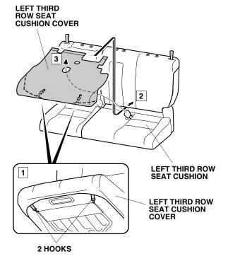
7. Secure the left third row seat cushion cover to the left third row seat cushion with the two hook-and-loop fasteners.
