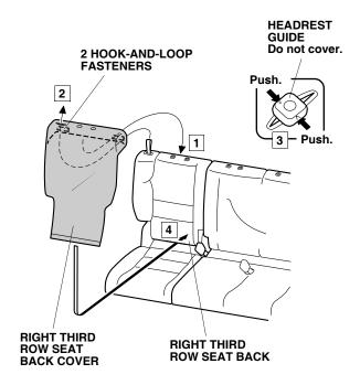
Fold down the right third row seat. Secure the right third row seat back cover to the right third row seat back with one hook-and-loop fastener. Return the right third row seat to its standard postion.
