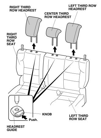
Push the knob and remove each headrest from the third row seats.  Install the two third row headrest covers and center third row headrest cover to three headrests as shown.
