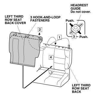
Fold down the left third row seat. Secure the left third row seat back cover to the left third row seat back with one hook-and-loop fastener. Return the left third row seat to its standard position.
