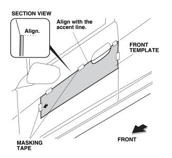
2. Peel back approximately 1½ to 2 inches of adhesive backing, and tape the ends to the front surface of the body side molding. Remove the small end pieces of adhesive backing.
