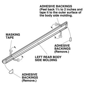
10. Clean the location where the left rear body side molding will attach with one alcohol swab.
