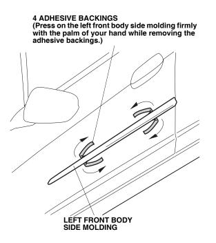
7. Using a rubber roller, apply firm pressure while rolling to set the adhesive.
