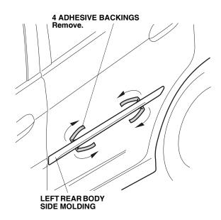
14. Using a rubber roller, apply firm pressure while rolling to set the adhesive.
