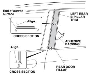
6. Using a rubber roller, apply pressure to set the adhesive.
