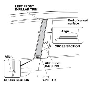
3. Using a rubber roller, apply pressure to set the adhesive.
