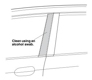
Peel back about 3 inches of adhesive backing from the left front B-pillar trim and fold it up diagonally as shown. Align the left front B-pillar trim on the left B- pillar as shown. While applying pressure on the trim, carefully remove the adhesive backing.
