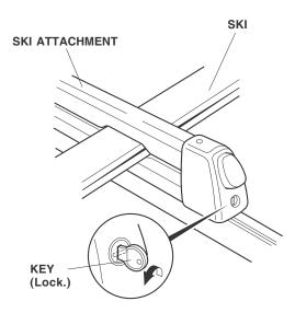
5. With the skis attached, rock the attachment in all directions to make sure it is installed securely. Adjust as necessary.
