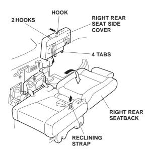
7. Unlock the right rear seat by pulling the right rear seat foot lock release strap out toward you.
