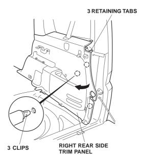
15. Remove and discard the cover from the right rear side trim panel. Slide the accessory socket protector into the vacant hole and align the tab on the protector with the cutout in the panel.
