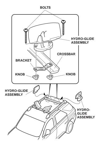
Rest the front of the kayak on the hydro-glide assemblies. Standing behind or alongside the kayak, lift up the rear of the kayak and push it forward onto the hydro-glide assemblies and saddles. Make sure the kayak reaches the front saddles before you lower it.
