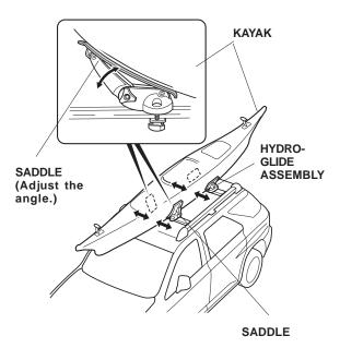
Slide the kayak forward or backward until it's level with the roof. If necessary, loosen the knob of each saddle and adjust the saddle angle to fit snugly against the kayak. Tighten each knob securely. 6. Route each strap with buckle through the buckle cover with the ribbed side facing up.
