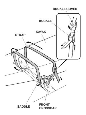
8. Route the strap under the rear crossbar, and around the kayak as shown. Slide the buckle cover away from the buckle, route the strap through the buckle, and tighten the strap. Slide the buckle cover back over the buckle.
