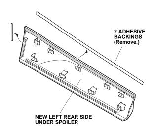
10. Hold the new left rear side under spoiler against the door, and install the trim seal to the door panel. Fit the nine clips into the holes in the body, then push on the side under spoiler until the clips snap into place.
