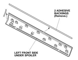
13. Hold the new left front side under spoiler against the door, and install the trim seal to the door panel. Fit the 13 clips into the holes in the body, then push on the left front side under spoiler until the clips snap into place.
