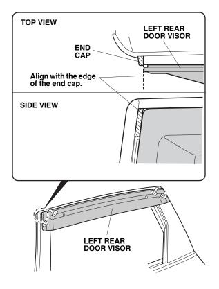
17. While holding the door visor up firmly, remove the adhesive backing in the order shown. Use your finger to push up each bracket so there is no gap between the brackets and the door sash.
