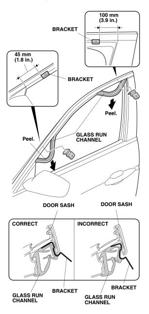
Install two brackets between the door sash and the glass run channel at the measurements shown.
