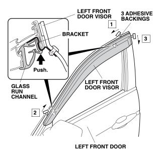
9. Using a soft towel, press and hold the left front door visor against the door for 30 seconds.
