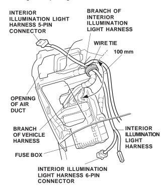
12. Measure the vehicle harness from the point of the branch as shown. Secure the interior illumination light harness (6-pin connector side) to the vehicle harness with one wire tie.
