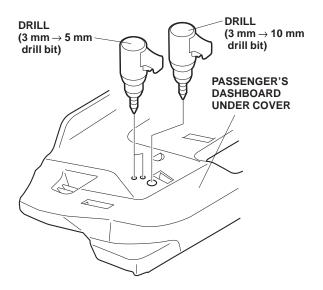
42. Route the interior illumination light (with white tape) connector through the 10 mm hole. Install the interior illumination light on the passenger's dashboard under cover with a screw and flange nut.
