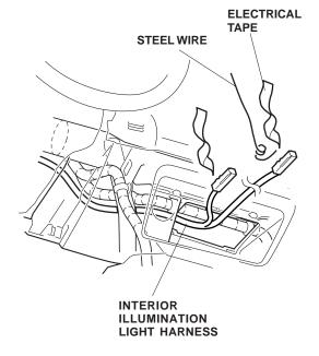
20. Remove the wire and electrical tape from the interior illumination light harness.
