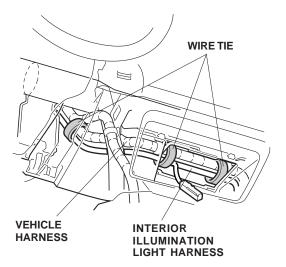
24. Secure the interior illumination light harness to the vehicle harness using four wire ties if the vehicle is equipped with the driver's dashboard under cover. Use three wire ties if the vehicle does not have a driver's dashboard under cover.
