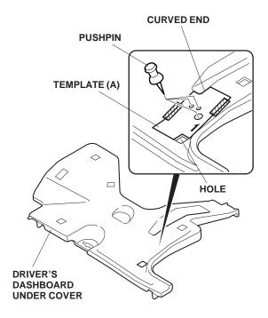
29. While wearing eye protection, drill one 10 mm hole and two 5 mm holes at the pierced points in the driver's dashboard under cover. First drill with a 3 mm bit, then finish with a 5 mm bit/10 mm bit as shown. Using a file, remove any burrs from the holes.
