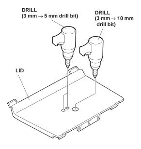
37. Route the interior illumination light (with blue tape) connector through the 10 mm hole. Install the courtesy light on the lid with a screw and flange nut.
