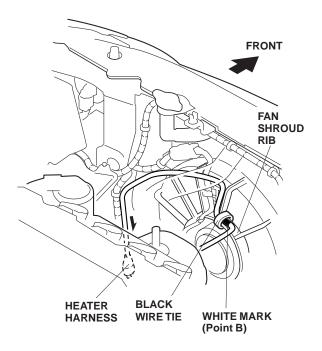
10. Secure the wire tie with clip, attached at point C, to the vehicle frame and route the heater harness to the front bumper opening.
