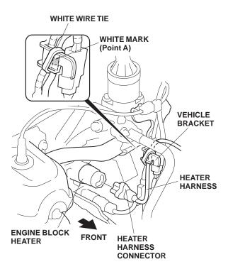
Secure the heater harness to the fan shroud rib with one black wire tie at the white mark (point B). Route the heater harness under the vehicle frame.
