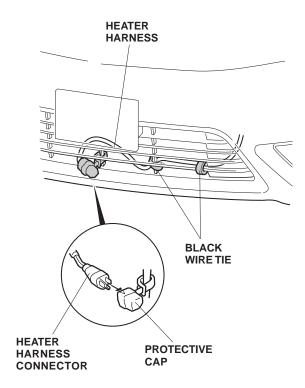
13. Attach the protective cap to the grille, and plug the connector of the heater harness into the protective cap.
