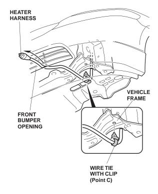
11. Secure the heater harness to the fan shroud rib and the vehicle harness using five black wire ties.
