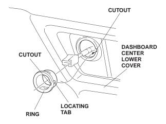
8. Connect the vehicle 2-pin connector to the socket.
