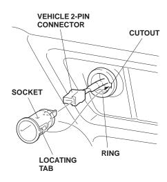
Align the locating tab on the socket with the cutout in the ring, and slide the socket into the ring. 10. Push the cigarette lighter into the socket.
