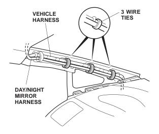
29. Plug the day/night mirror harness 6-pin connector into the 6-pin connector at the fuse box.
