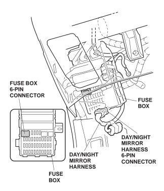
NOTE: If another accessory is already plugged into the 6-pin connector, remove the dummy connector from the 6-pin connector taped to the day/night mirror harness. Disconnect the 6-pin connector of the other accessory harness from the fuse box and connect it to this 6-pin connector.
