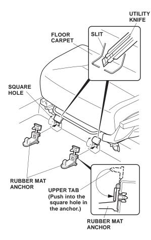
3. Push the lower tab of the anchor into the square hole concealed under the floor carpet. Pull the upper tab down, and push it into the square hole in the anchor as shown. Repeat on the remaining anchor.
