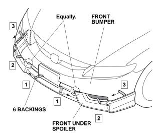
30. Using a rubber roller, apply firm pressure while rolling to set the adhesive.
