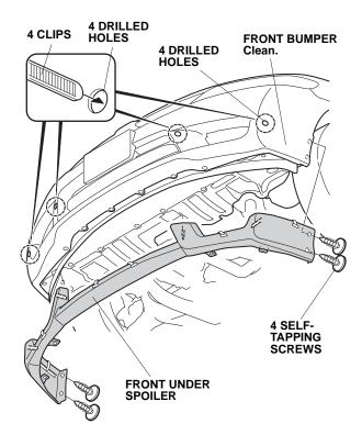
22. Position the front under spoiler on the front bumper, and loosely install four self-tapping screws as shown.
