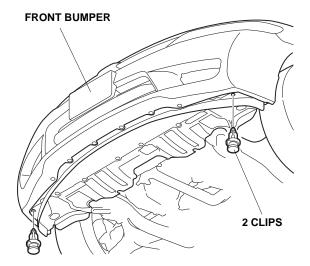
19. Attach one sponge seal to each clip on the front under spoiler as shown.
