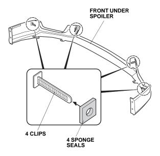
20. Attach a strip of masking tape to the end of each backing, and peel back 30 to 40 mm of the backings. Fold the ends back, and tape them to the front of the front under spoiler.
