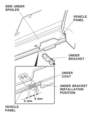
25. Cut into the marked area of the undercoat with a utility knife, and file off the undercoat from both sides of the vehicle panel.
