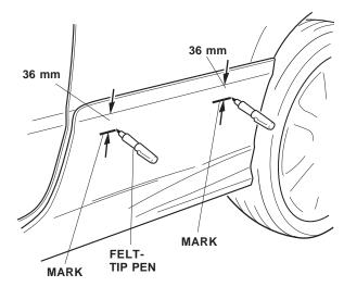
37. Using isopropyl alcohol on a shop towel, clean the area where the sticker will attach. Attach the sticker to the side under spoiler at the marks you made in step 36. Align the corner of the sticker to the rear edge of the side under spoiler.
