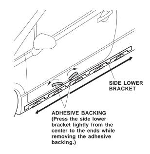
When the ambient temperature is below  $60^{\circ}F$  (15°C), warm up the entire side lower bracket to  $60^{\circ}F$  (15°C) or above before attaching it to the vehicle body.
