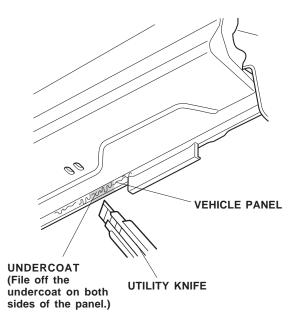
26. Apply touch-up paint to the vehicle panel in the area where you filed off the undercoat. Do not install the under bracket until the touch-up paint dries.
