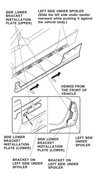
23. Check that all six brackets on the left side under spoiler are set in the side lower bracket installation plates. Visually check that there is no excessive gap between the left under spoiler and the vehicle. If an excessive gap is found, repeat step 22. 24. Fit the under bracket to the side under spoiler and mark the undercoat.
