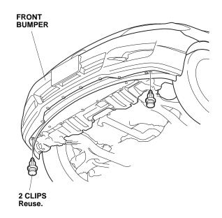
20. Attach one sponge seal to each clip on the front under spoiler as shown.
