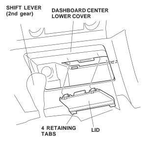
Open the accessory socket cover. Using a shop towel around a small flat-tip screwdriver, gently pry on the accessory socket to pop it out. Disconnect the vehicle 2-pin connector from the accessory socket.
