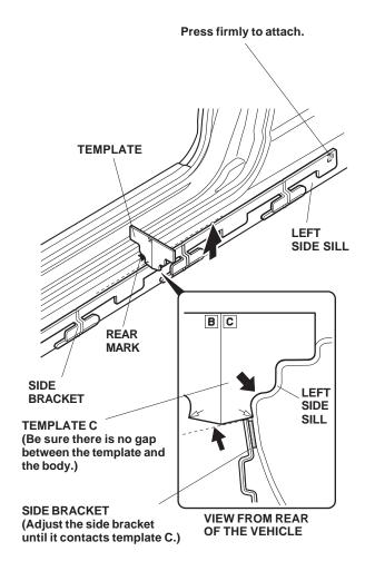
10. While wearing gloves, press the rear portion of the side bracket (where you removed the adhesive backing) firmly against the vehicle body so that the adhesive will adhere.
