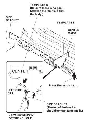
14. While wearing gloves, press the center portion of the side bracket (where the adhesive tape was peeled back) firmly against the vehicle body so that the adhesive will adhere.
