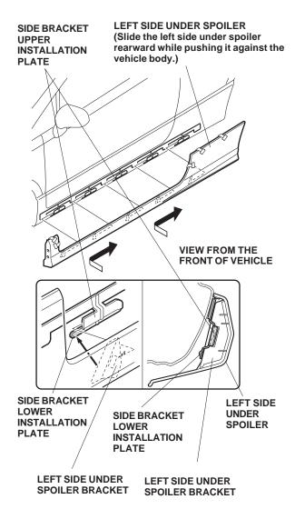
21. Check that all six brackets on the left side under spoiler are set in the side bracket installation plates. Visually check that there is no excessive gap between the left under spoiler and the vehicle. If you can see a gap, repeat step 20.
