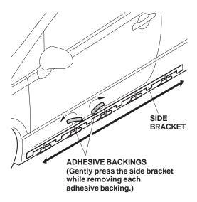
16. While wearing gloves, attach the side bracket to the vehicle body by pressing firmly along the double-sided adhesive tape with the palms of your hands.
