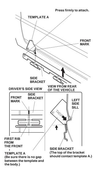
12. While wearing gloves, press the front portion of the side bracket (where you removed the adhesive backing) firmly against the vehicle body so that the adhesive will adhere.
