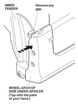
25. Loosely install the front self-tapping screws in the holes in the wheel arch of the side under spoiler.
