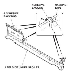
20. Check the position of the under spoiler attachments by looking down at them from the top. While pushing the left side under spoiler against the vehicle body with both hands, slide it rearward. Make sure the location of the side bracket installation plates (upper and lower) attach to the brackets on the under spoiler.
