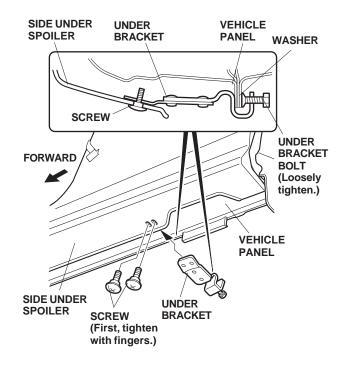
27. Position the under bracket on the side under spoiler and loosely install the two screws. Loosely tighten the under bracket bolt.
