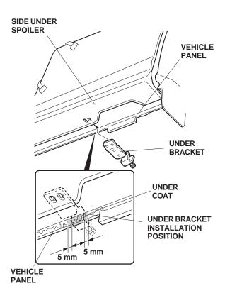
23. Using a utility knife, cut the undercoat at the marked location, and file off the undercoat from both sides of the vehicle panel.
