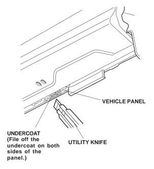
24. Apply touch-up paint to the vehicle panel in the area where you filed off the undercoat. Allow the touch-up paint to dry.
