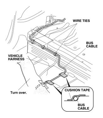
27. Secure the bus cable to the vehicle harness with three wire ties in the areas shown.
