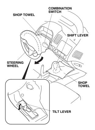
7. To protect the dashboard area, place shop towels over the steering wheel and shift lever.
