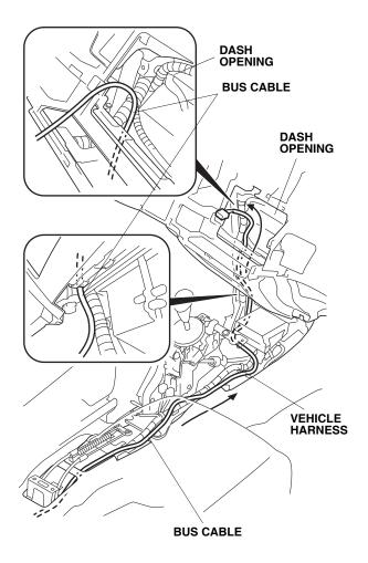
22. Continue routing the bus cable to the dashboard and out through the dash opening.
