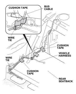
29. Using isopropyl alcohol on a shop towel, clean the areas where the cushion tapes will attach. Attach the bus cable to the floor panel with three cushion tapes in the areas shown.
