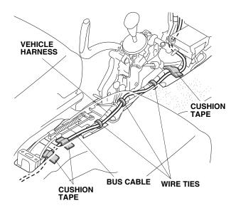
25. Using isopropyl alcohol on a shop towel, clean the areas where the cushion tape will attach. Attach the bus cable to the floor panel with the three cushion tapes in the area shown.
