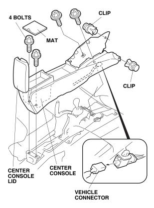
13. Remove the center console (four bolts and two clips, and unplug the vehicle connector).
