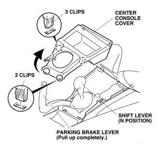
12. Open the center console lid, and remove the mat.
