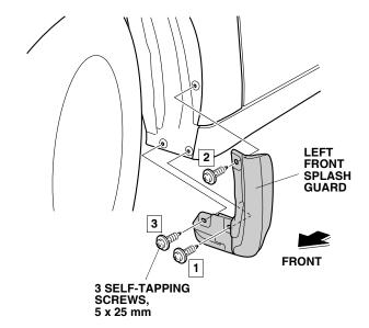
8. Secure the left front splash guard to the driver's side sill trim with one clip.
