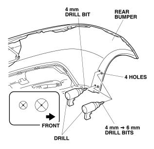
16. Enlarge the two front holes on the rear bumper with a 6 mm drill bit. Remove any burrs.
