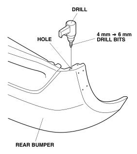
15. Drill the four holes on the rear bumper with a 4 mm drill bit.
