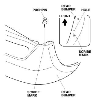
14. While wearing eye protection, drill the hole on the rear bumper with a 4 mm drill bit, then enlarge the hole with a 6 mm drill bit. Remove any burrs.
