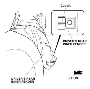
21. Install one spring nut to the hole on the driver's rear inner fender.
