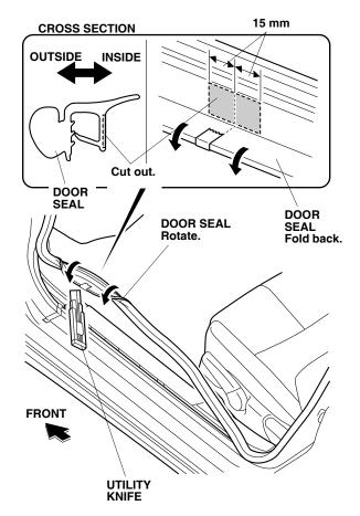
17. Using a utility knife, make a slit in the door seal rubber to expose the small metal plates inside the rubber seal.
