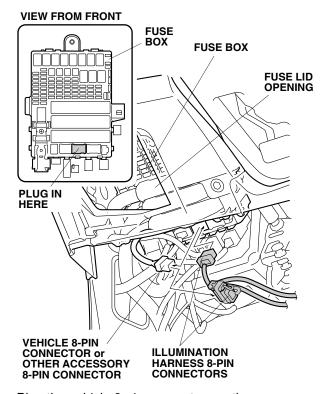
Plug the vehicle 8-pin connector or other accessory 8-pin connector into the illumination harness 8-pin connector. 39. Route the illumination harness 2-pin connector down, and plug it into the left illuminated door sill trim 2-pin connector.
