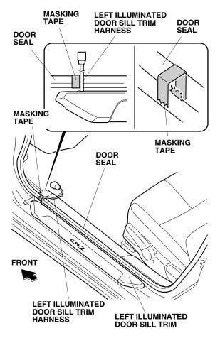
13. Route the left illuminated door sill trim harness over the door seal, and attach a piece of masking tape to the door seal to mark the illuminated door sill trim harness location.
