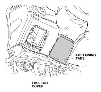
6. Remove the driver's under cover (turn the knob, two clips, and one pin).
