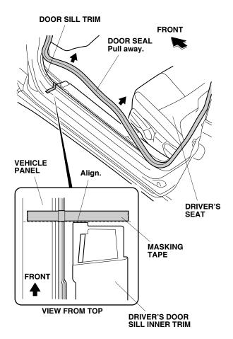
Attach a piece of masking tape to the vehicle panel even with the front edge of the driver's door sill inner trim. 11. Align the left illuminated door sill trim with the masking tape.
