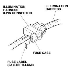
37. Unplug the vehicle 8-pin connector or other accessory 8-pin connector (if equipped) from the fuse box, and plug the illumination harness 8-pin connector into the fuse box.
