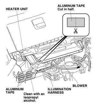
51. Using scissors, cut one aluminum tape in half.
