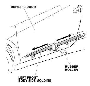
14. Press the body side molding firmly with the palm of your hand, and remove the adhesive backings.
