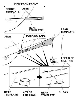
6. Align and attach the rear template to the body panel with masking tape.
