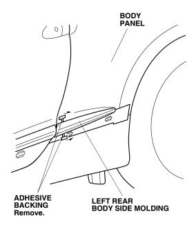
15. Using a rubber roller, apply pressure against the body side molding and roll from one end to the other.
