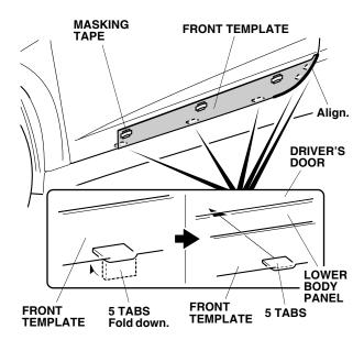
4. Align and attach the front template to the driver's door with masking tape.
