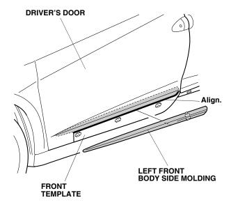
9. Peel back approximately 1½ to 2 inches of adhesive backing from each adhesive tape, and tape the ends to the front surface of the body side molding.
