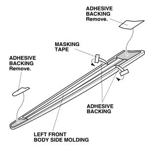
8. Align the left front body side molding with the front template, and attach it to the driver's door.
