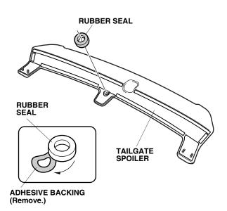
17. Open the tailgate and install the spoiler on the tailgate. Install the four cap nuts to the spoiler studs and torque the cap nuts to 8.8 N·m (6.5 lb-ft).
