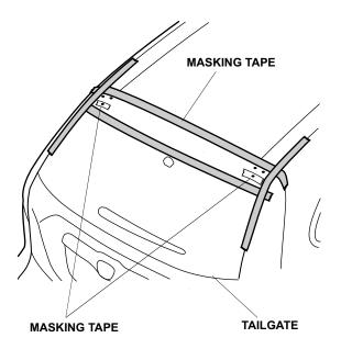
7. Open the tailgate. Apply masking tape over the ends of the taillight housing. Close the tailgate.
