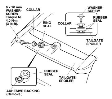
19. Install the collar and 6 x 20 mm washer-screw through the rubber seal and into the tailgate spoiler. Torque the 6 x 20 mm washer-screw to 4.0 N⋅m (3 lb-ft).
