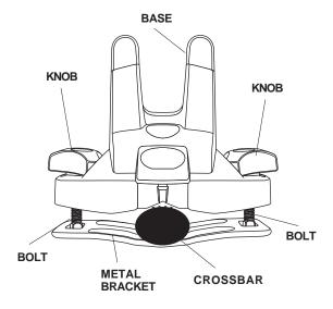
3. Repeat steps 1 and 2 for the three remaining bases. Install two bases on each crossbar.
