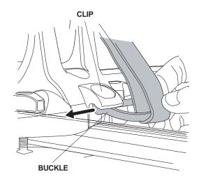
7. Rotate the buckle up to "lock" it into the base. Repeat this step at the remaining bases.
