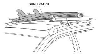
Adjust the position of the bases so that the bottom of the surfboard rests on the rubber part of the bases. Tighten all knobs firmly and evenly.
