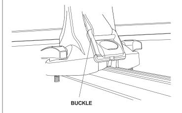
8. Pull the ends of the attachment straps to secure the surfboard to the carrier. Make certain all mounting hardware is secure, then tighten as necessary.
