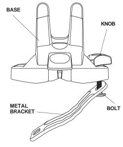
Position the base on the crossbar. Loosely install an additional bolt and knob through the metal bracket.
