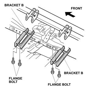
19. Secure brackets A and B together using eight flange bolts and eight 8 mm flange nuts.
