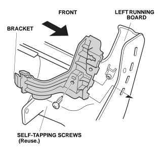
14. Remove the two spring nuts from the left side sill panel and install them on the left running board in the areas shown.
