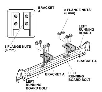
17. Position the left running board on the vehicle, and secure both brackets A using four flange bolts. Make sure the inner fender fits on the inside of the left running board end cap. Align the clips installed in step 15 to the holes in the body panel, and push them into position.
