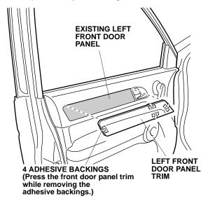
15. Repeat steps 12 thru 14 to install the door panel trim on the remaining three doors.
