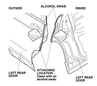
12. Using a spray bottle with 3M protective tape application solution, spray the outer surface where the left rear door edge films will attach.
