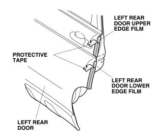
19. Starting from the center and working outward, use the applicator to fold the left rear door upper edge film and left rear door lower edge film inside the left rear door as shown. Move in one direction only. Do not damage the door seal during this procedure.
