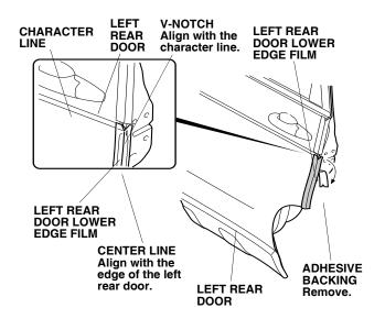
16. Align the center line on the left rear door lower edge film with the edge of the left rear door. While applying light pressure, carefully remove the adhesive backing, and attach the left rear door upper edge film to the left rear door.
