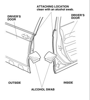
2. Close the driver's door. Using a spray bottle with 3M protective tape application solution, spray the outer surface where the left front door edge film will attach.
