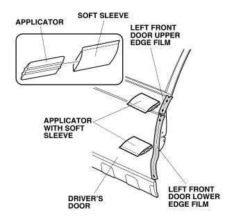
8. Slowly remove the protective tape from the left front door upper edge film and left front door lower edge film.
