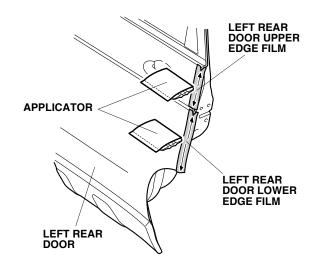
18. Slowly remove the protective film from the left rear door upper edge film, and left rear door lower edge film.
