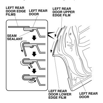
20. Using a shop towel, wipe up the excess 3M protective tape application solution from the door edge film. Allow the left rear door edge film to dry thoroughly.
