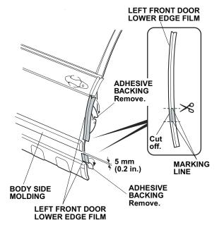
6. Align the center line on the left front door edge film with the edge of the left front door. While applying light pressure, carefully remove the adhesive backing and attach the left front door lower edge film to the driver's door.
