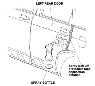
Open the left rear door. Peel back about 50 mm (2 in.) of adhesive backing from the left rear door upper edge film. Align the V-notch with the end of the character line on the upper part of the left rear door as shown.
