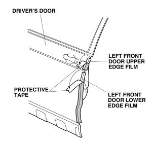
9. Starting from the center and working outward, use the applicator to fold the left front door upper edge film and left front door lower edge film inside the driver's door as shown. Move in one direction only. Do not damage the door seal during this procedure.
