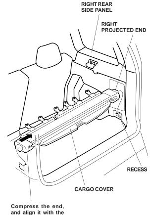
and align it with the recess in the left rear side panel.
