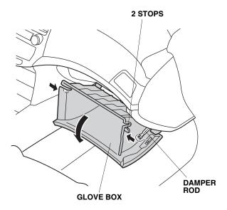
10. Remove the glove box (two screws).
