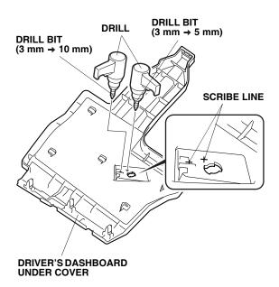
Using an utility knife, cut out the driver's dashboard under cover as shown.
