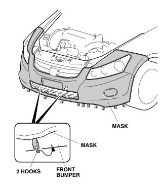
14. Attach four plastic hooks to the inside edge of the front bumper.
