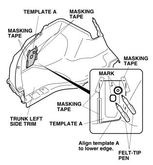
7. Using a felt-tip pen, mark the trunk left side trim as indicated on the template. Remove the template.
