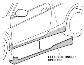
2. Open the door. Position template A on the vehicle body. Using a felt-tip pen, mark the vehicle body at the distance shown.
