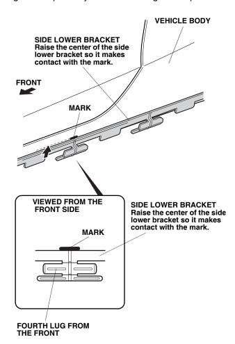
13. Make sure the side lower bracket makes contact with the marks. Apply pressure to the side lower bracket starting from the center and moving to the ends while removing the adhesive backing that was temporarily attached to the lower bracket.
