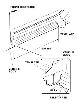
4. Position template C on the vehicle body. Using a felttip pen, mark the vehicle body at the distance shown.
