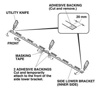
6. Attach a piece of masking tape to each of the cut ends as shown, and temporarily attach them to the front of the side lower bracket as shown.
