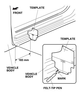
3. Position template B on the vehicle body. Using a felttip pen, mark the vehicle body at the distance shown.
