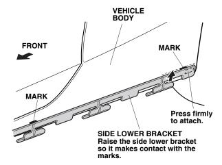
Verify the alignment, then press the front end of the side lower bracket (where you removed the adhesive backing) to attach the part firmly to the vehicle body.
