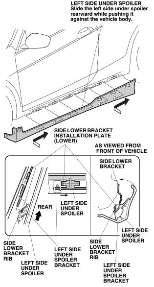
20. Check that all six brackets of the left side under spoiler are set in the side lower bracket installation plates. Visually check that there is no excessive gap between the left under spoiler and the vehicle. If an excessive gap is found, repeat step 19.
