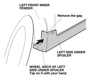
22. Loosely install two 5 x 18 mm self-tapping screws in the holes in the wheel arch of the left side under spoiler.
