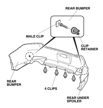
22. Secure the rear under spoiler to the rear bumper using four 5 x 14 mm self-tapping screws and four plain washers as shown.
