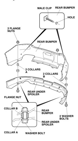
21. Secure the rear under spoiler to the rear bumper using four clips and two clip retainers as shown.
