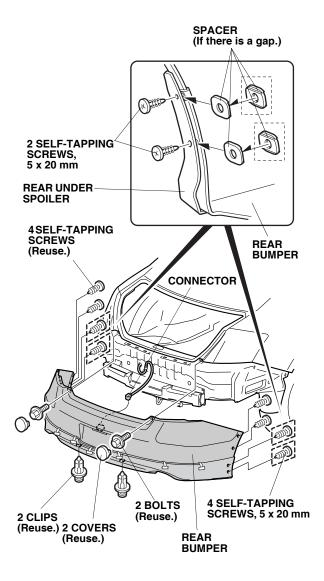
25. While applying pressure on the rear under spoiler, carefully remove the adhesive backings from the center outwards. After removing the adhesive backings, hold the rear under spoiler firmly against the rear bumper with the palm of your hand for 30 seconds. Apply pressure to the bumper from the inside of the rear under spoiler and outside of the rear under spoiler with your hands as shown.
