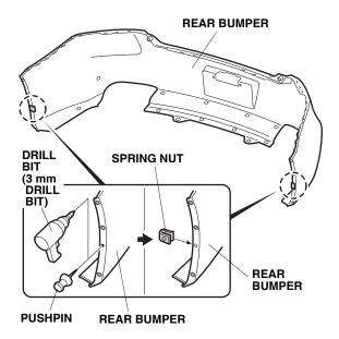
10. Slide two spring nuts over two holes you made in the rear bumper.
