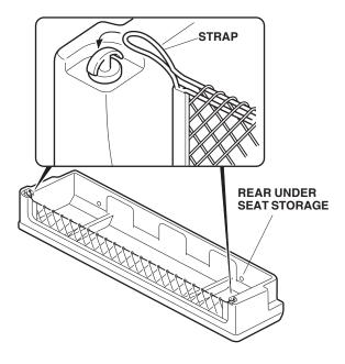
6. Position the rear under seat storage on the floor mat, and align the holes in the rear under seat storage with the holes in the brackets. Secure the seat storage with the two knob bolts.
