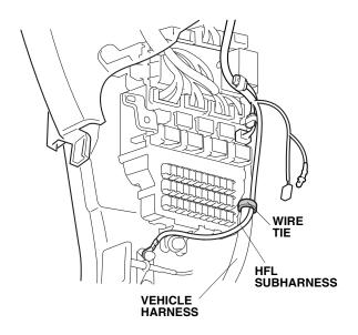
22. Route the HFL subharness as shown, and secure it to the vehicle harness with one wire tie.
