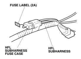
18. Plug the HFL subharness 6-pin connector to the 6-pin opening on the fuse box.
