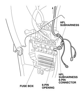
19. If other accessory is already plugged into the 6-pin connector, remove the dummy connector from the 6-pin connector taped to the HFL subharness. Plug the other accessory 6-pin connector into the HFL subharness and plug the HFL subharness into the fuse box.
