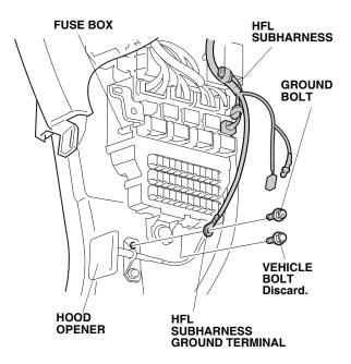
21. Secure the HFL subharness to the vehicle harness with one wire tie.
