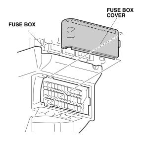
66. Install the 2A fuse into the No.33 slot of the fuse box.
