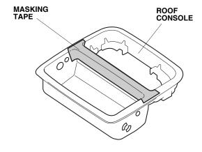
39. Attach template A to the roof console at the indicated position with masking tape.
