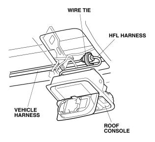
64. Plug the vehicle connectors to the roof console. Reinstall the roof console with four screws removed in step 5.
