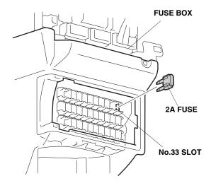
67. Attach the fuse label (OPTION FUSE 2A) to the No.33 on the inside of the fuse box cover.
