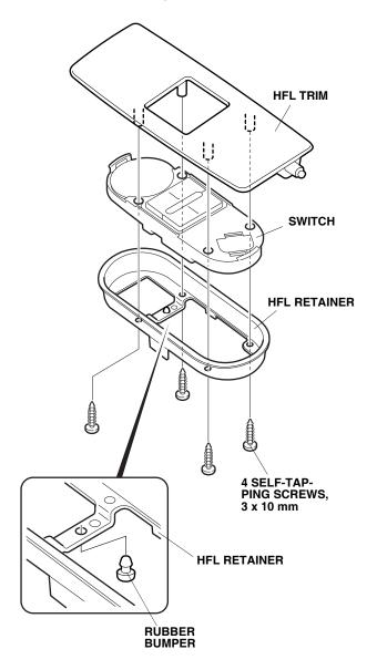
56. Assemble the HFL retainer, switch, and HFL trim with four 3 x 10 mm self-tapping screws.
