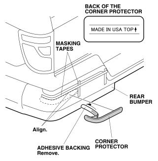
16. Attach the corner protector to the rear bumper by aligning it with the masking tapes as shown.
