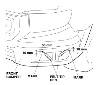
3. Align and attach the masking tapes to the marks made on the front bumper.
