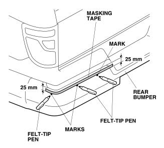
11. Align and attach masking tape to the marks made on the rear bumper.
