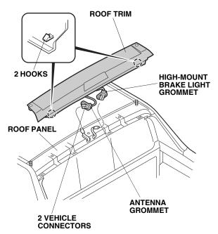
37. Remove the antenna grommet and high-mount brake light grommet from the roof panel, unplug the vehicle connectors, and remove the roof trim.
