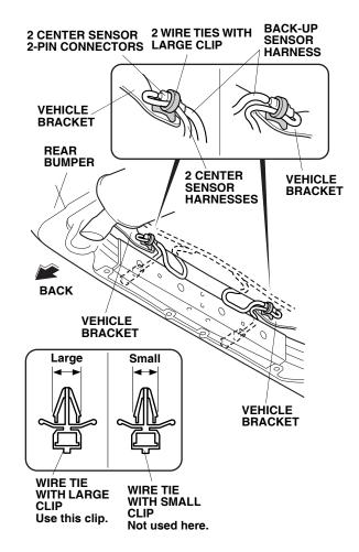
88. Inside of the vehicle, turn over the floor mat, and route the back-up sensor harness across the vehicle panel and alongside the vehicle harness.
