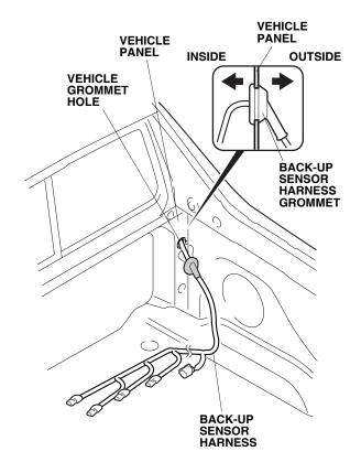
74. Inside the cargo area, route the back-up sensor harness along the vehicle harness, and secure the front of the back-up sensor harness to the hole on the vehicle panel with one wire tie with small clip. Align the wire tie with small clip to the green tape on the back-up sensor harness as shown.
