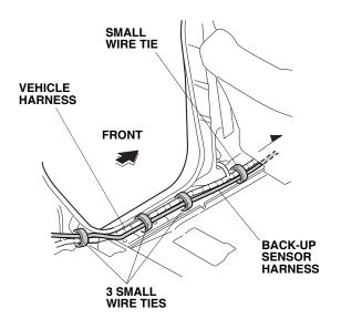
98. Route the back-up sensor harness along the vehicle harness, and secure it to the vehicle harness with three small wire ties.
