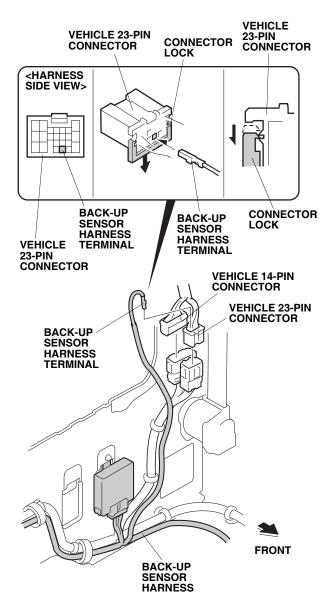
95. Push the back-up sensor harness terminal into vehicle 23-pin connector, then reattach the connector lock. Re-plug the vehicle 23-pin and 14-pin connectors.
