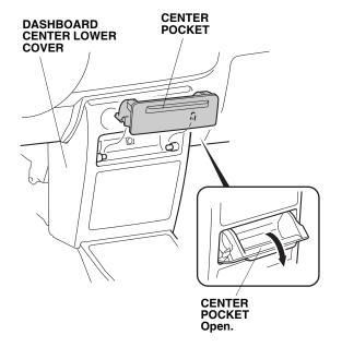
8. Remove the dashboard center lower cover (three self-tapping screws, five clips, six retaining tabs, and unplug the vehicle connectors).
