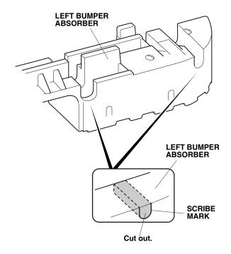
57. Remove the left and right bumper absorber. Locate the scribe mark on the left bumper absorber. Using an utility knife, measure and cut out the left bumper absorber along the scribe mark as shown. Repeat the same procedure for the right bumper absorber.
