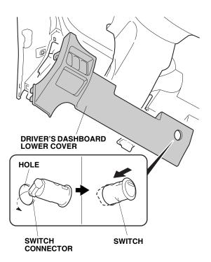
109. Plug the back-up sensor harness 3-pin connector into the switch.
