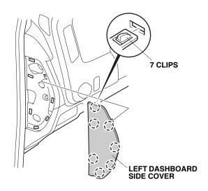
4. Remove the driver's dashboard lower cover (one self-tapping screw, nine clips, unplug the vehicle connectors, and the vehicle tube).
