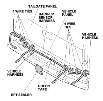
83. Using isopropyl alcohol on a shop towel, clean the area where the EPT sealer will attach. Secure the back-up sensor harness to the vehicle panel with one EPT sealer at the green tape.
