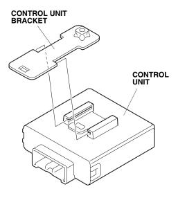
93. Plug the back-up sensor harness 22-pin connector into the control unit, and insert the control unit bracket into the hole on the vehicle panel. Secure the control unit bracket with one flange bolt.
