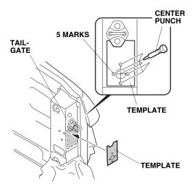
62. While wearing gloves and eye protection, drill one 26 mm hole and four 8 mm holes through the marked locations. First drill with a 3 mm drill bit, then finish the center hole with a 26 mm hole saw and the outer holes with an 8 mm drill bit.
