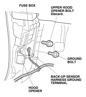
100. Route the back-up sensor harness as shown, and secure it to the vehicle harness and the vehicle frame with six wire ties.
