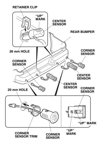
59. Separate the corner sensors from the corner sensor trims. First install the corner sensor trim into the 20 mm holes with the "UP" mark facing up, then install the corner sensors through the corner sensor trim with the "UP" mark on the sensor facing up.
