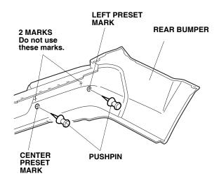
55. While wearing eye protection, drill one 20 mm hole through the outer mark, and one 26 mm hole through the inner mark on the rear bumper. First drill with a 3 mm drill bit, then finish the outer hole with a 20 mm hole saw and finish the inner hole with a 26 mm hole saw. Remove any burrs. Repeat the same procedure for the right side.
