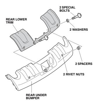
12. Secure the rear lower trim to the rear under bumper with four bolts and two clips.
