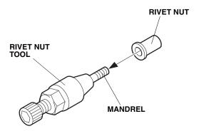
• Insert the rivet nut into the hole in the rear under bumper and install the hex wrench on the rivet nut tool.
