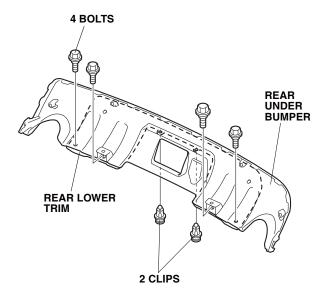
13. Reinstall the rear under bumper to the rear upper bumper.
