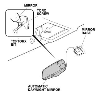
9. Plug the automatic day/night mirror harness 7-pin connector to the automatic day/night mirror. Route the automatic day/night mirror harness as shown.
