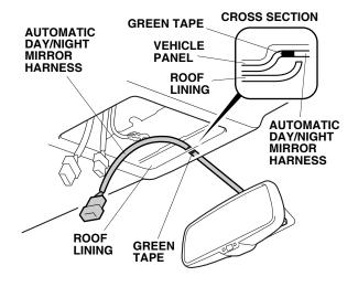
11. Locate the vehicle 6-pin connector and remove a blue tape from the vehicle 6-pin connector. Plug the automatic day/night mirror harness 6-pin connector to the vehicle 6-pin connector.
