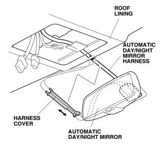
15. Bring the harness cover to be in contact with the roof lining.
