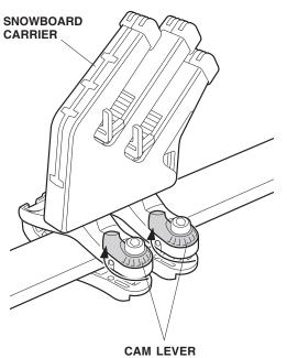
CAM LEVER Return to their original positions. 10. To prevent theft, install the screws in the holes in the top clamps using a TORX wrench.
