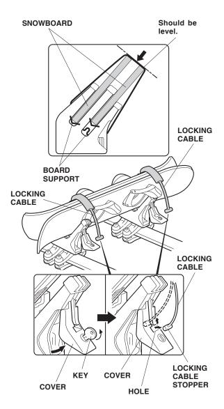
Check that the plate is inserted in the slot securely. Check that the locking cable is inserted in the groove securely.
