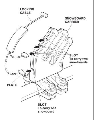
15. After loading the snowboards on the carrier, adjust them with the help of the board supports so that the top edges are level and the boards are as far down in the carrier as possible. To secure the snowboards, use the key to open the covers and insert the locking cable stoppers into the holes of the carrier covers.
